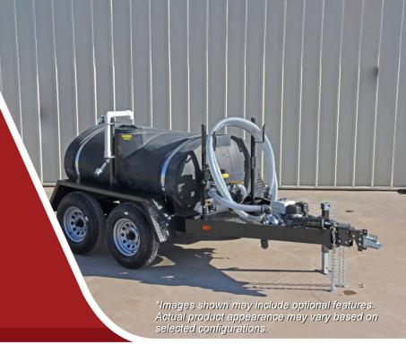
The 550 Gallon Potable Water Trailer is designed to safely transport clean drinking water to remote locations like RV parks, job sites, cabins, or events. Built with NSF/ANSI certified components and a black, algae-resistant poly tank, it ensures water purity from fill to discharge. A powerful Honda engine drives a stainless steel pump, providing reliable, high-flow transfer wherever water is needed.
