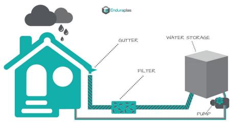
**Catchment surface** - The catchment surface is simply the first point of contact for rainfall. For many homeowners, this will be the rooftop due to the large square footage at your advantage. Your roof must have gutters to easily collect the rainwater at the storm drain. However, more factors go into discovering if your roof is optimal for rainwater harvesting.
